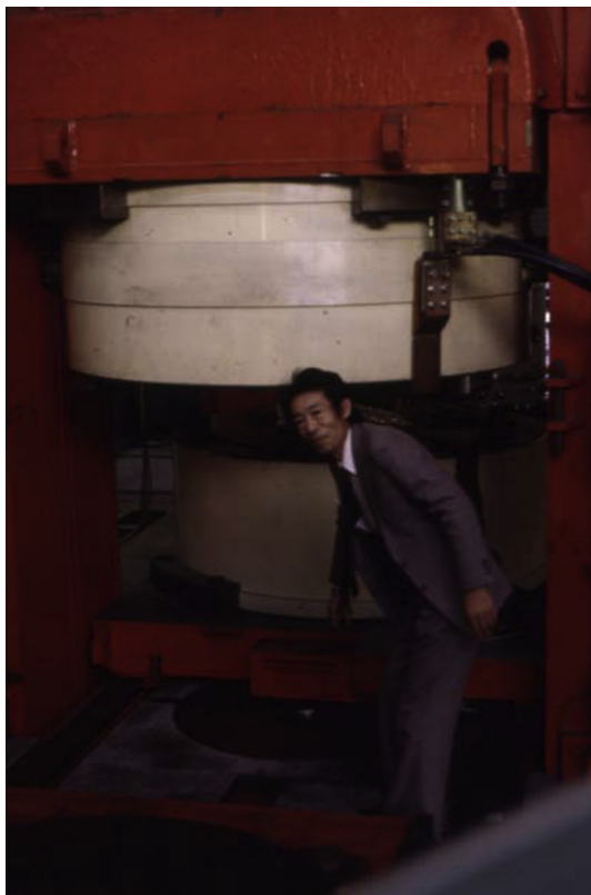
Fig. 5e. Mineo Kumazawa with 17,000 ton hydraulic press used to drive his newly designed multiple-anvil-sliding-system [MASS] at Nagoya University.
